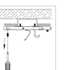
Remove the 4 preassembled screws from mounting plate (Corresponding to installation step 8). Save screws for later use.
