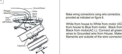
White from house to White from motor (AC N)Blue from house to Blue from motor. Black from house to Black from motor(AC L). Connect all green grounded wires to Grounded wire from House. Make sure that no filaments are outside of the wire connector.
