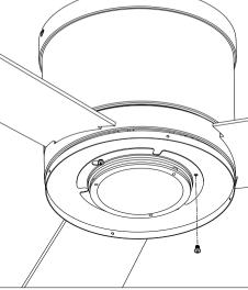
Installing the LED assembly Loosen two screws and remove one screw on the light kit. Attach light kit to the light kit mounting plate using three screws provided.
