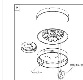
Installing the center band and blade
