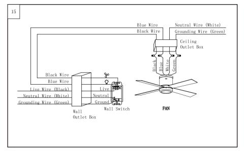
Make wire connections using wire nuts:
