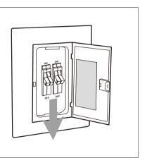
power off at Service panel and lock service disconnecting means to prevent power from being switched on accidentally. When the service disconnecting means cannot be locked. securely fasten a warning device, such as a tag, to the service panel.
