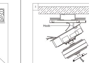
Before you begin installing the fan, Switch Before installing this fan make sure the outlet box is properly installed to the house structure. To reduce the risk of fire, electric shock, or personal injury. mount to outlet box or supporting system acceptable for fan support. (Mounting must support at least 35 lbs.)
