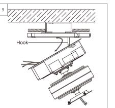
Hang motor assembly onto the hook on mounting plate for hands-free wiring
