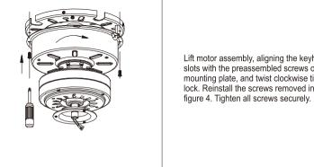
Lift motor assembly, aligning the keyhole slots with the preassembled screws on mounting plate, and twist clockwise till lock. Reinstall the screws removed in
