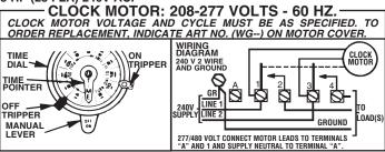
WIRING INSTRUCTIONS: To wire switch follow diagram above. Use solid or stranded COPPER only wire with insulation to suit installation. See gauge selection table for normal service applications. To make power connections remove 1/2 inch of insulation from wire ends. Insert bare ends of wire under the pressure plate of terminals. Use 3/16 or larger screwdriver to tighten terminal screws firmly. (25 lb-in minimum).
