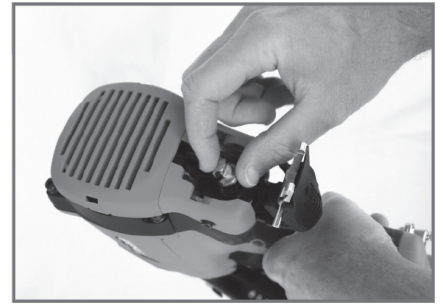
Carefully align fuel adaptor and cell stem
