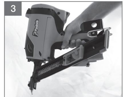
3 Gently release follower onto rear of nail strip, to prevent collation damage
