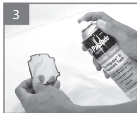
3 Cleaner/Degreaser or soap and water restores the filter
