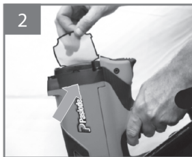
2 Tap filter gently against hard surface to remove dust
