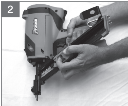
2 Depress lever, then pull nail follower back past nail strip
