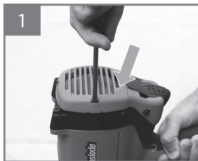
1 Use a flat bladed screwdriver to remove cap
