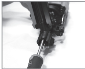
Push or punch the driver blade back to top rest position, using a long punch (if needed)
