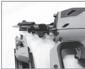
Remove the magazine assembly to expose the back of the nose slot. (Be careful the nail follower does not come out of the magazine channel)
