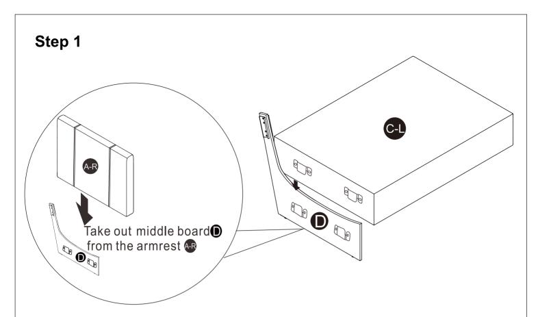
Please put PART "D" on the ground and lift the seat frame to inset into PART "D".
