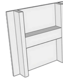
Wall studs with blocking
