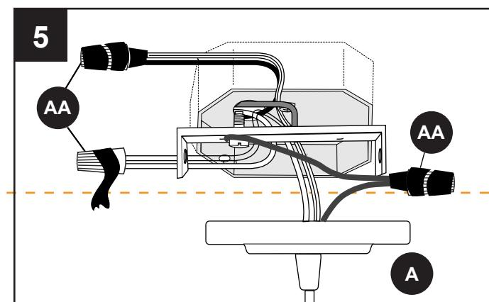
**⚠ Make sure no bare wire or wire strands are visible after making connections.**
