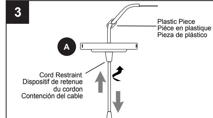
**OPTIONAL:** Loosen plastic piece (do not remove) and cord restraint to change cord length. Pull cord up through canopy of A. Tighten cord restraint to hold cord at desired length.
