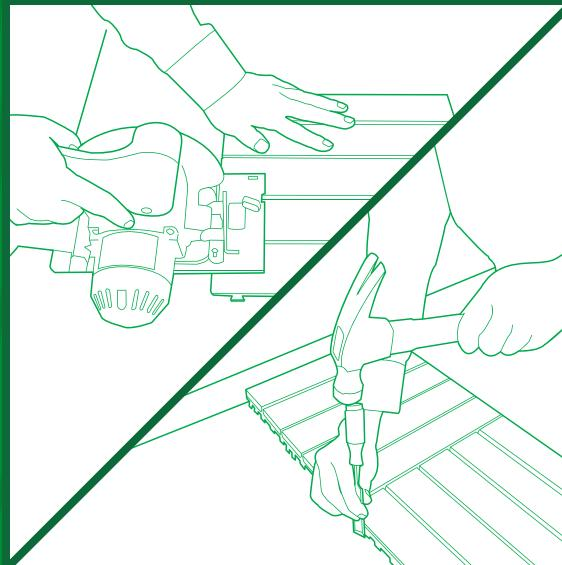
Using a circular saw (16 teeth or less) cut tile to the desired length. Make quick cuts. A chisel can be used to remove exposed connectors where transition pieces are not used. Loose boards may be secured using 1/2" long, #8 screws (not included), installed through the small round holes on the back of the tile.
