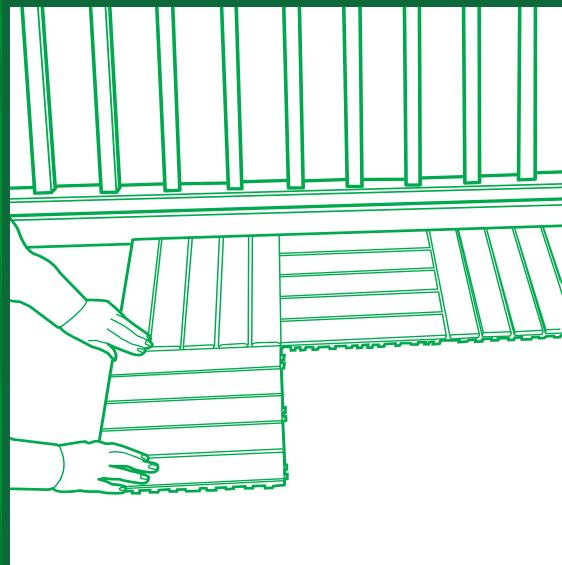
Lay tiles starting at outside edge of surface. This ensures that cut tiles are the last row against the house, fence, pool, etc. Continue laying tiles and snapping them together using checkered or parallel patterns until desired surface is covered.
