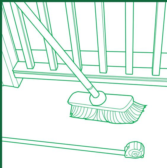
Clean the solid surface of all debris to ensure proper water drainage. To determine the number of tiles you will need, first measure the area to be covered. If measuring in feet, multiply by 12 to convert to inches, then divide by 11.8 to determine the number of tiles needed.
