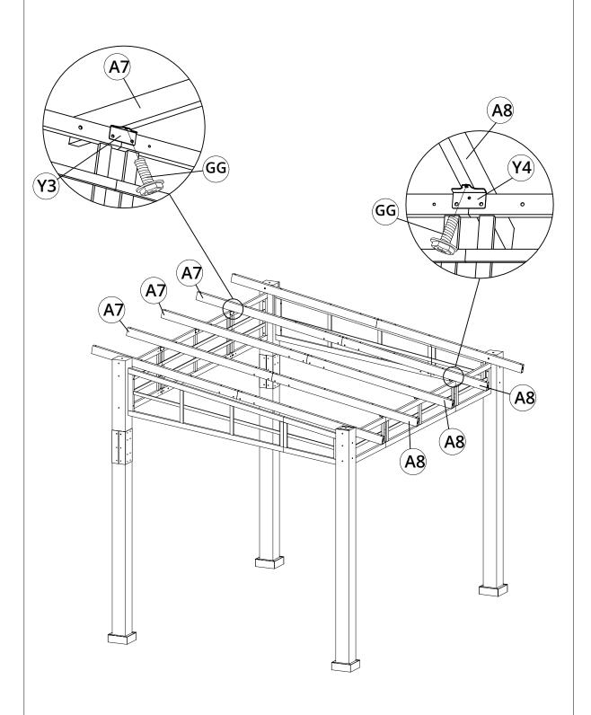
Note: A7 A8 parts do not need to be locked tightly for subsequent installation
