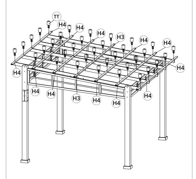
Note: H3 H4 parts do not need to be locked tightly for subsequent installation
