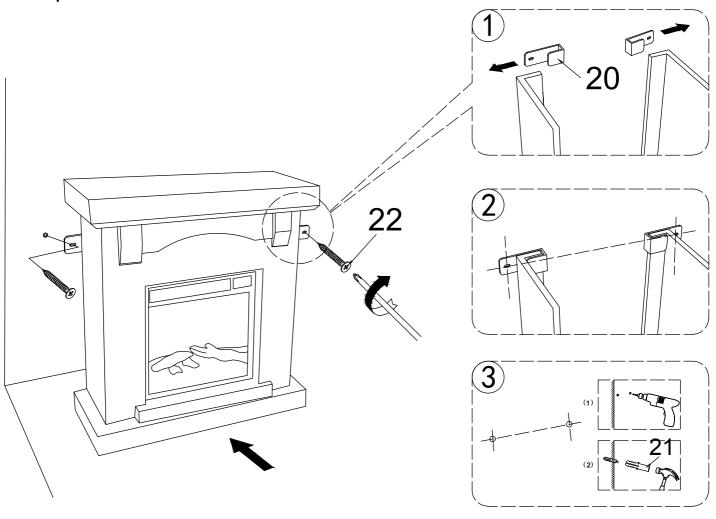
Install the Anti-tipping Brackets (20) from the back of the fireplace. Secure the Brackets (20) by using the M4x30mm screw (22) and the Plastic Anchor (21).
