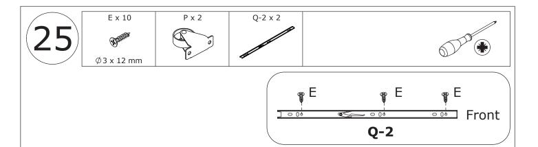
Fix runner(Q-2) and wheel(P) to plate 26 and 27 with screw(E) as shown.
