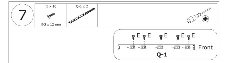
Separate glide into two parts at first(turn to page 7). Fix slide rail(Q-1) to plate 15 and 16 with screw(E) as shown.
