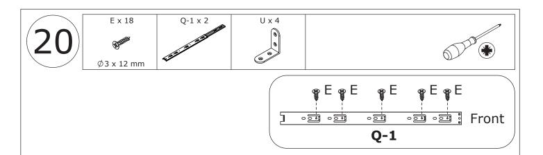
Fix rail(Q-1) and part(U) to plate 22 and 23 with screw(E) as shown.
