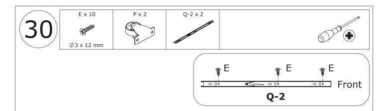
Fix runner(Q-2) and wheel(P) to plate 29 and 30 with screw(E) as shown.
