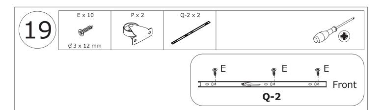
Fix runner(Q-2) and wheel(P) to plate 22 and 23 with screw(E) as shown.
