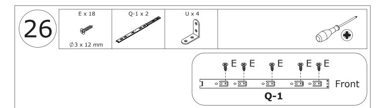
Fix rail(Q-1) and part(U) to plate 26 and 27 with screw(E) as shown.
