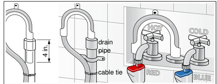
Attach the drain hose to the elbow included with your washer.
