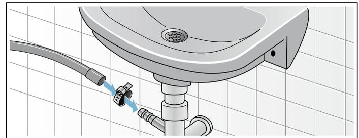
Secure the drain hose to the sink siphon using a  $\varnothing$  0.9 - 1.6 in. (20-44 mm) hose clip (available from a hardware store).
