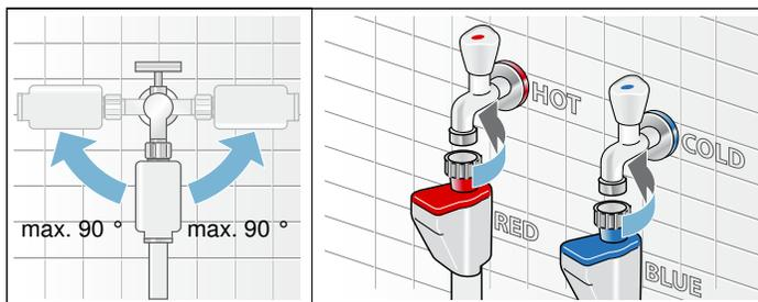
**Attach this end to water tap.** Hand tighten only.
