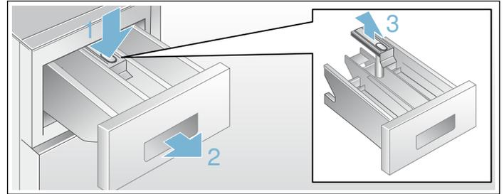
1. Open the detergent dispenser tray fully. Press down on the drawer catch (1) and pull the tray (2) from the washer housing.
