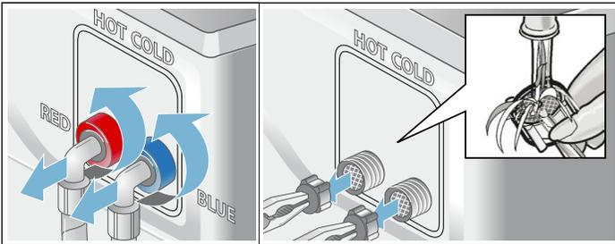
1. Remove the hose from the inlet on the back of the washer.
