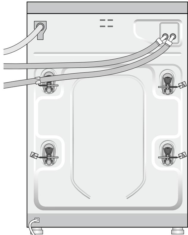
Position hoses as shown when routing hoses to left side of washer (facing from front).
