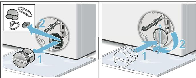
6. Turn the pump cover counterclockwise to remove it. A small amount of residual water may flow out when the cover is removed. Clean the interior of the pump housing, removing any debris or foreign objects. Check to be sure the impeller wheel at the back of the pump housing can now turn freely. Remove any lint, debris or detergent residue from the threads of the pump cover and the pump cover housing. Replace the pump cover by screwing tightly into position. Handle must be vertical.
