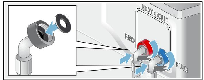
**Attach this end of the hose to the back of the washing machine as shown in the following pictures. Be sure to use clamps and route hoses as instructed.** Hand tighten only.
