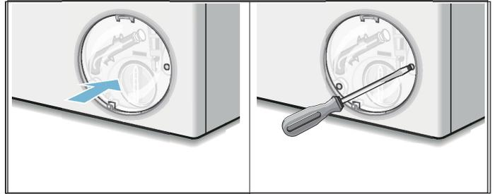
8. Snap the service cover in place at the hinges and close it. Wipe up any spilled water.
