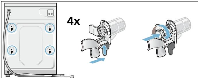
1. Each assembly consists of a plastic bushing and a bolt that extends through the bushings. Unscrew the bolt until the threaded end is flush with the end of the plastic bushing.
