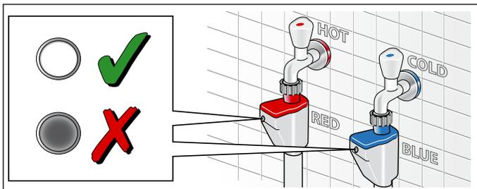
The AquaShield® hose prevents potential flooding in the event the hose develops an internal leak. If the hose leaks, the indicator turns red and water flow is blocked. Once the internal valve in the hose activates (indicator is red) the hose must be discarded. Contact customer service for a replacement.
