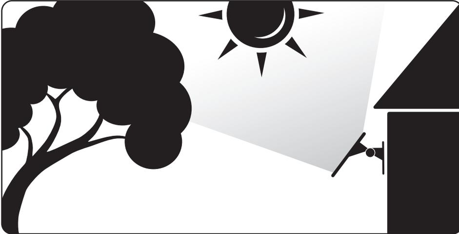
Mount the solar panel facing due south with direct line of sight to the sun. Be sure to avoid any potential obstructions, such as buildings or trees, that may cast a shadow on the panel during the day.
