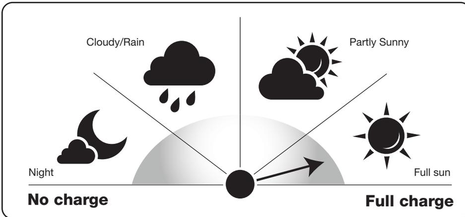
All solar panels require consistent, unobstructed exposure to the Sun to perform at their best. Any clouds, rain, pollen or dust etc. may increase the amount of time it takes the batteries to recharge. Use a mild detergent to wipe the panel clean whenever necessary.
