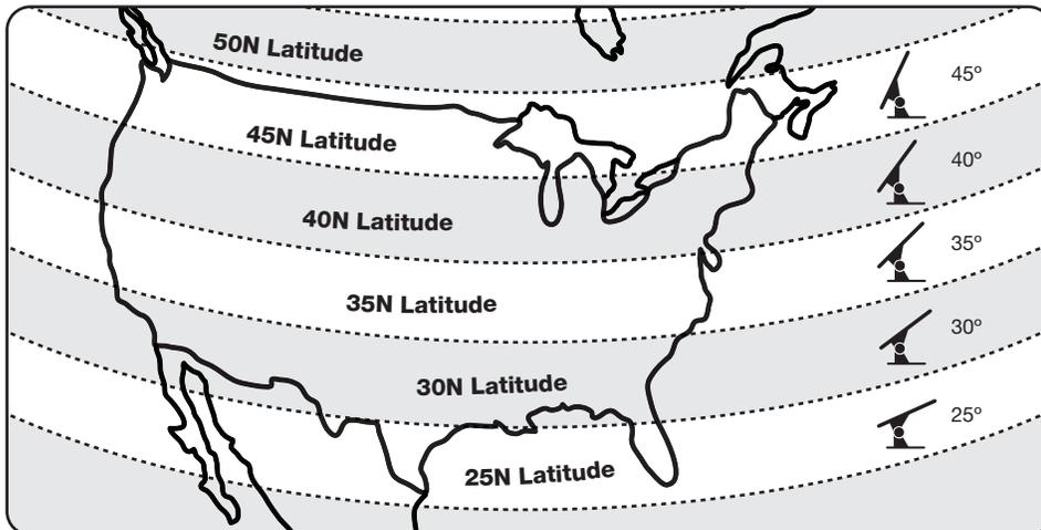
Orient the solar panel at approximately the same angle as the latitude of your location, taking into consideration the angle of the surface you are mounting it to.
