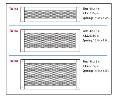
The opening should be *at least* 1 inch smaller than the vent size.
