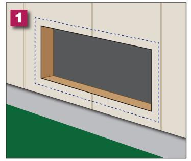
1. Remove old vent and any loose debris from opening.
