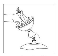
Remover the R-pin and Cross pin from downrod.Thread the wires through the downrod, and insert the Downrod into the Couple. Hanger ball Canopy Downrod Cover R pin Setscrew Coupler Coupler
