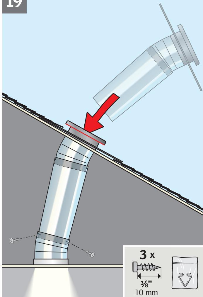
**ENGLISH:** Connect tunnel assembly with the clips supplied. If tunnel section was trimmed or holes do not align, use the screws supplied as necessary.
