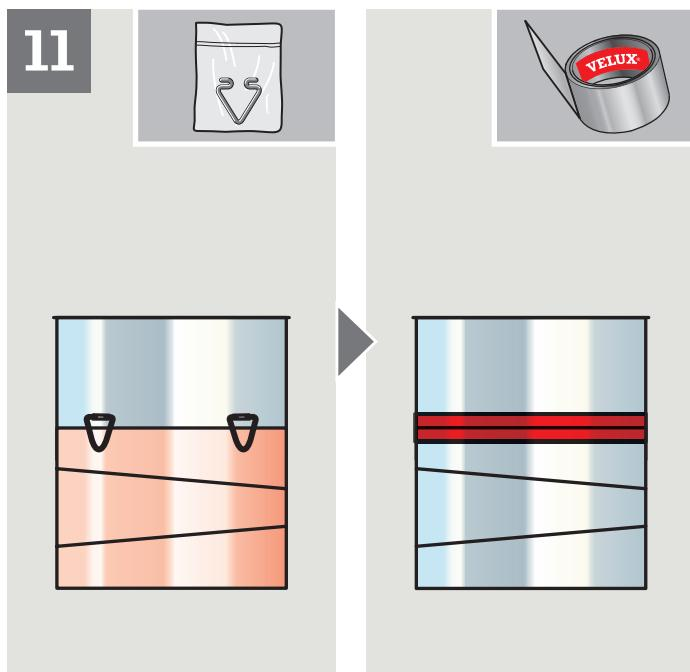
**ENGLISH:** Attach the upper elbow to the top collar. Secure joints with tunnel clips and tape provided.
