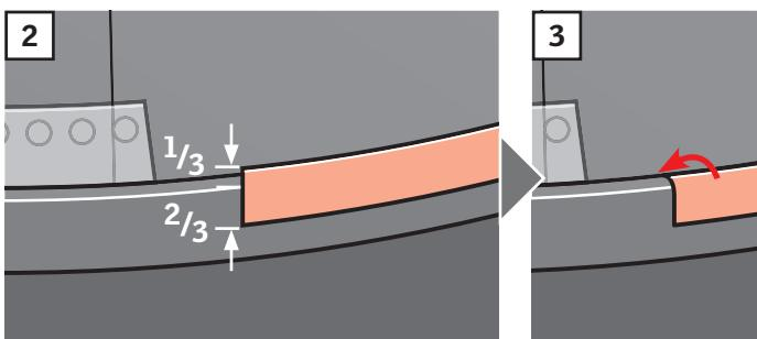
**ENGLISH:** in order to conform to Hallmark certification, foam tape must be applied over drainage holes **1** and around and over edge of frame **2**, **3** as shown.
