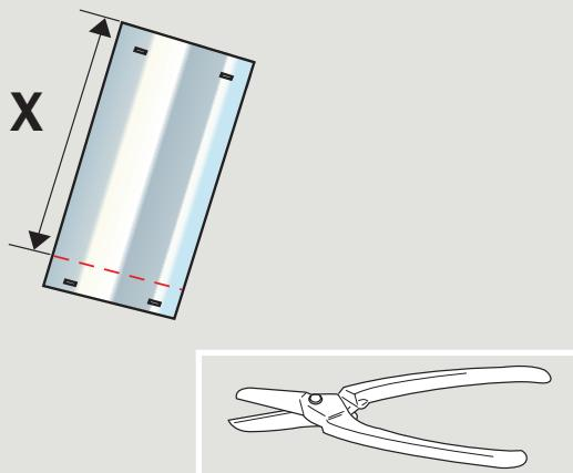
**ENGLISH:** With one rigid tunnel section, cut the section to length.
