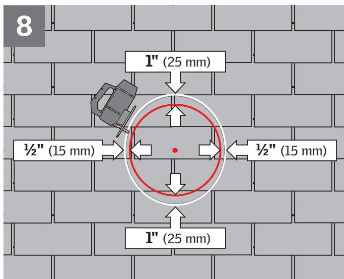
**ENGLISH:** Mark and cut a rough opening of  $\frac{1}{2}$ " (15 mm) outside the circle at the sides and 1" (25 mm) outside the circle at top and bottom.
