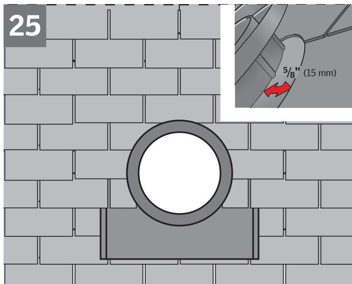
**ENGLISH:** Reinstall roofing material over the flange. Leave a  $5/8"$  (15 mm) channel for water to run off.
