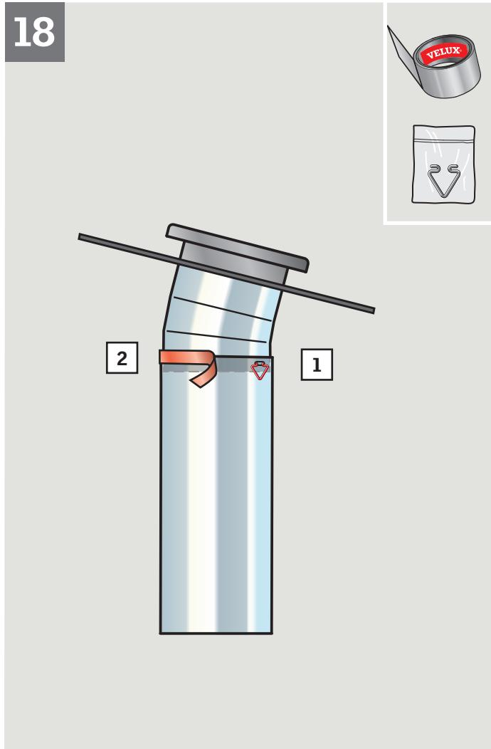
**ENGLISH:** Connect the rigid tunnel section with upper elbow, fitting the rigid tunnel section to go on the outside of the upper elbow. Secure and tape joints with tunnel clips and tape provided **1, 2**.
