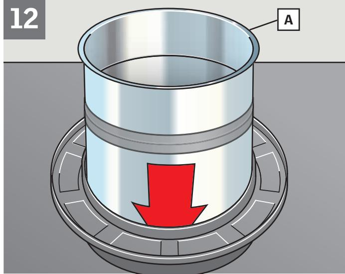
**ENGLISH:** Insert the upper elbow into the flashing allowing the retaining edge **A** to rest on the flashing.
