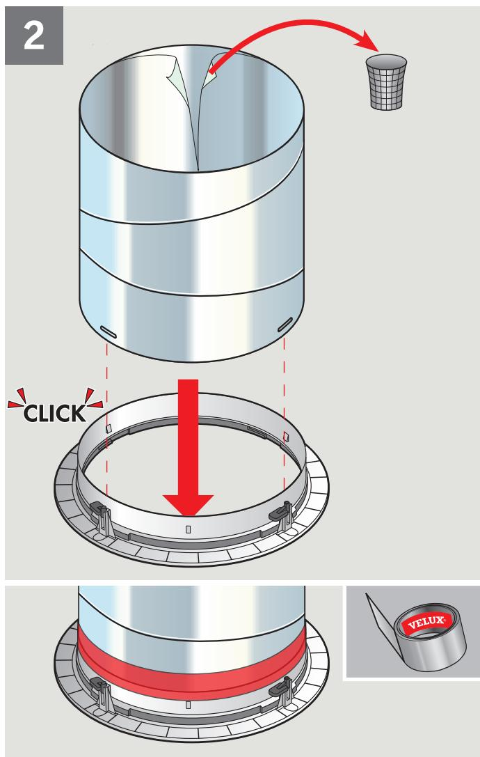
**ENGLISH:** Attach lower elbow to the ceiling ring. Make sure all ceiling ring tabs engage with a click. Remove protective film from the lower elbow. Tape joint between lower elbow and ceiling ring.
