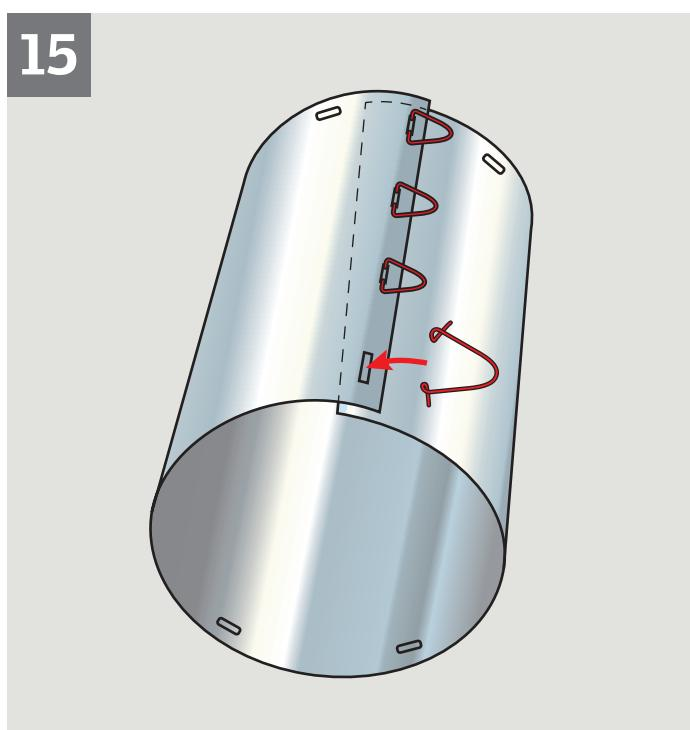
**ENGLISH:** Assemble the rigid tunnel section with tunnel clips provided.
