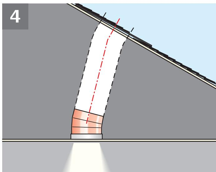
**ENGLISH:** Adjust the angle of the lower elbow. When it is positioned correctly, it will be in line with the upper elbow. Elbows can be damaged if excess force is applied. Refer to the illustration for optimal positioning.
