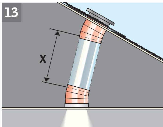
**ENGLISH:** Adjust the angle of the upper elbow so that it points directly against the lower elbow. Elbows can be damaged if excess force is applied.
