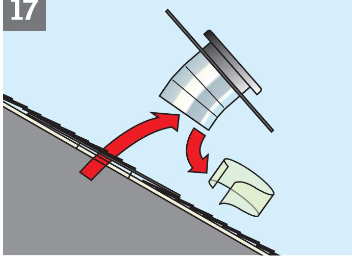
**ENGLISH:** Remove flashing with elbow and remove protective film from upper elbow.
