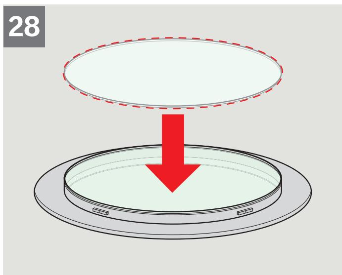
**ENGLISH:** Install the secondary diffuser disc onto the primary diffuser.
