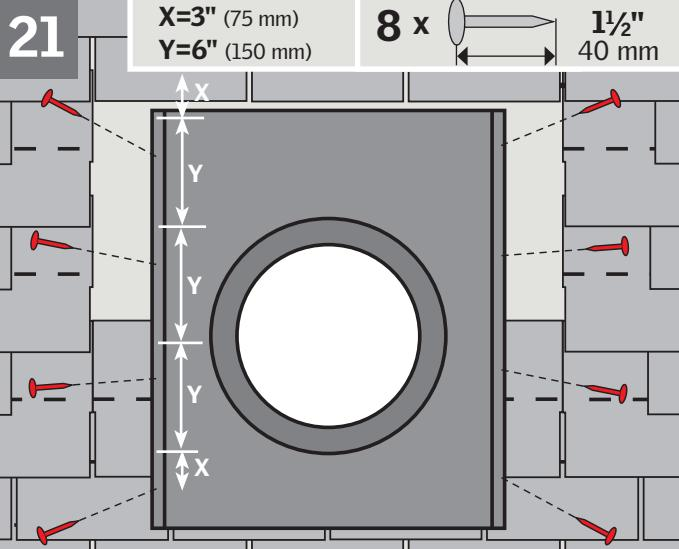
**ENGLISH:** Center the flashing over the rough opening and secure the flange with nails along the sides. Seal all exposed nail heads.
