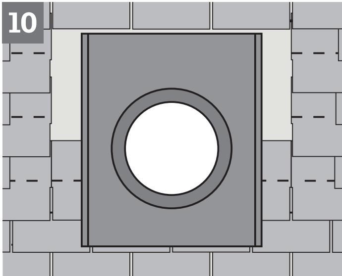
**ENGLISH:** Temporarily install the flashing over the rough opening.
