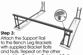
end of the Benches. Tighten all Bolts and Nuts securely.
