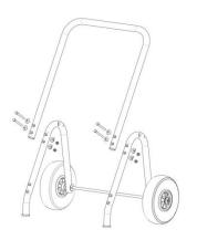
5. Use the rubber pad (item 13), washer (item 12), and the knobs (item 11) to assemble the heater to the foot stand. Tighten the knobs as
