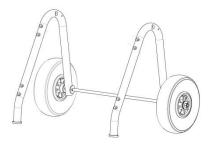
4. Use the screw (item 10), washer (item 9), and nut (item 8) to assemble the handle to the foot stand as shown below. Tighten the nuts.
