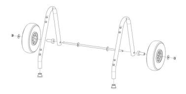
3. Tighten the nuts (item 6) to the wheels as shown below:
