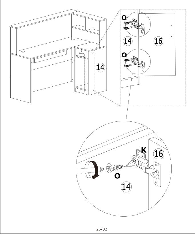
If there is misalignment after you install, adjust the screw to the best condition
