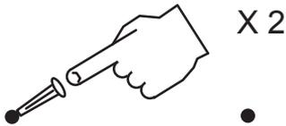
**2** Drill into the wall at each marked location. Use a 1/4" drill bit for brick or other masonry wall. Use a 1/16" drill bit for wood wall.
