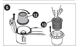
If necessary, wash the two filters (12 and 13) in warm, soapy water.
