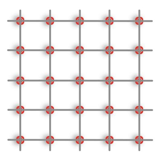
For our 3" rebar chair, we recommend placing a chair at every rebar crossing. Simply snap the bottom piece of reinforcement into the bottom clip, then snap the top piece of reinforcement into the top clip, and you are finished. No wire tying needed. Our rebar chair ensures the reinforcement stays in the right place before, during, and after the concrete pour.
