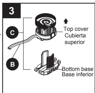
4. Insert wire from low-voltage transformer (sold separately) into the bottom base of connector (C) and then re-tighten the top cover removed in step 3 until the contact pins completely pierce the plastic shield of the wire.
