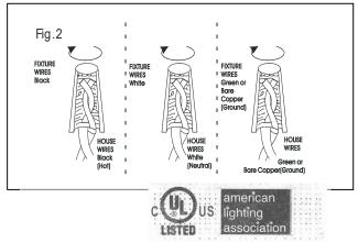
CAUTION-RISK OF FIRE. CONSULT A QUALIFIED ELECTRICIAN TO ENSURE CORRECT BRANCH CIRCUIT CONDUCTOR. MIN 90°C SUPPLY CONDUCTORS.
