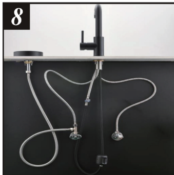
8. Choose cold or hot water for your glass rinser. Unthread existing faucet supply line from angle stop on the chosen side. Thread provided tee onto angle stop with wrench. Thread both the faucet supply line and the 3/8" end of provided supply line to tee. When supply line is installed check alignment and retighten mounting nut.
