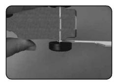
2. Slide an wheel adjustment tool between the wheel and body. Move the wheel until the tool fits snugly.
