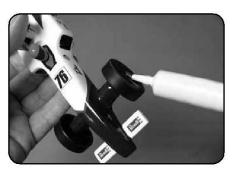
4. Apply graphite powder between the axle head and wheel. "Work in" the powder by shaking the car and slowly turning the wheel.
