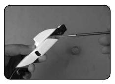
1. Remove all dust. Apply a thin coat of paint. When dry scuff lightly with fine sandpaper. Repeat as needed. Do not scuff the final coat.
