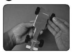
1. Place a wheel on all four axles. Press them into the axle slots.
