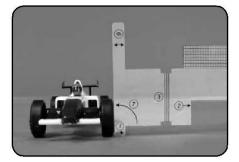
**3.** Put car on a smooth, flat surface. Put camber check section of tool against each wheel. Adjust each axle until the wheel is parallel to the tool.
