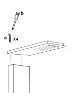
Put the shower head arm into panel body, then tightening the screws
