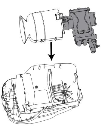
**Install the detergent tank** Secure detergent tank with (4) M6 screws
