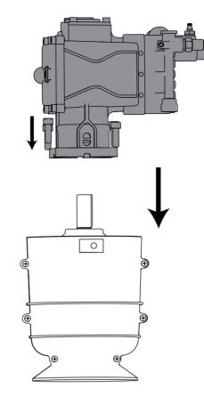
Install the lower bracket Secure lower bracket with (1) M8 screws and (4) ST5.5 screws
