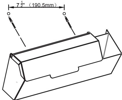
For brick or other masonry walls, insert the anchor into the wall. Install screws, ensuring to leave a gap of  $\frac{1}{4}$ " between wall and screw head. Anchors are not needed for a wood wall.
