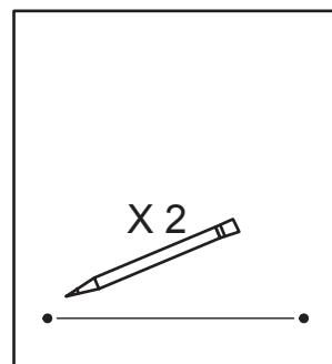
Using the template, mark screw holes. Check with level before drilling. Then, drill two 7/32" pilot holes (for masonry wall) or drill two 3/32" pilot holes (for wood wall, no anchors needed).
