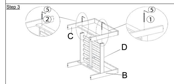
With assistance from your adult partner(s), attach the Left Leg Panel (C) to the assembled parts in Step 2 using Screws (1), Screws (2) and the Allen Wrench (5) as pictured
