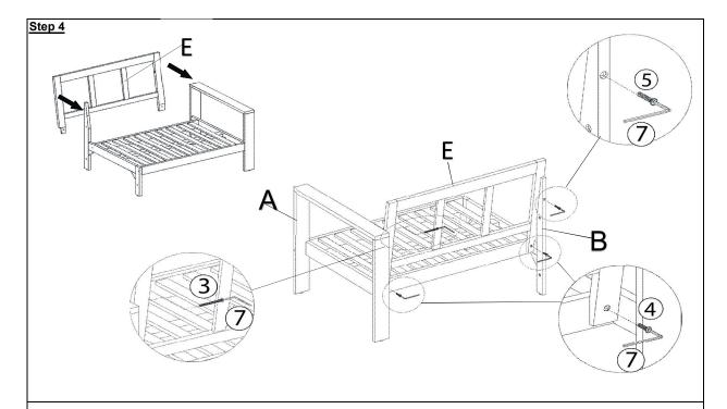
With assistance from your adult partner(s), attach the Right Backrest Panel (E) to the assembled frame in step 3 by using Bolts (3), Bolts (4), Bolts (5) and the Allen Wrench (7) as shown above.
