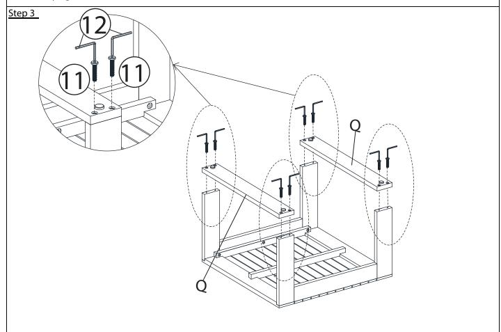
Attach the Base Leg (Q) to into the frame of step 2 by using Bolts (1), and Allen Wrench (2) as shown in picture above.
