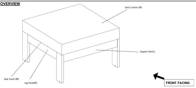
This Ottoman has multiple parts and may require up to some 30 minutes to assemble. To give you an overview of the Ottoman parts, the above picture is to help you put the various parts into perspective. Please read through the instructions below to familiarise youself with the parts and steps before assembly.
