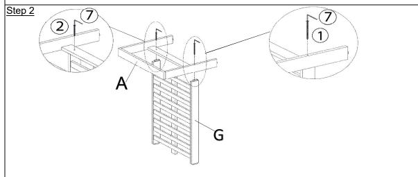
Place the Right Seat Panel (G) upright as shown in the picture above onto a clean, soft surface to avoid any scratches or damage to the product.
