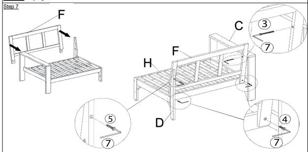
With assistance from your adult partner(s), attach the Left Backrest Panel (F) to the assembled frame in step 6 by using Bolts (③),Bolts (④), Bolts (⑤) and the Allen Wrench (⑦) as shown above.
