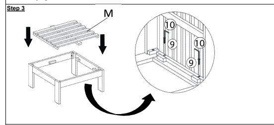
Insert the Seat Panel(M) into assembled Ottoman frame as pictured above.
