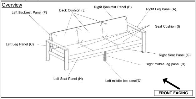
This 3 Seater has multiple parts and may require up to 60 minutes to assemble. To give you an overview of the 3 Seater parts, the above picture is provided to help you put the various parts into perspective. Please read through the instructions below to familiarise yourself with the parts and steps before assembly.
