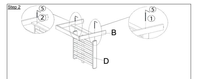
Place the Seat Panel (D) upright as shown in the picture above onto a clean, soft surface to avoid any scratches or damage to the product.
