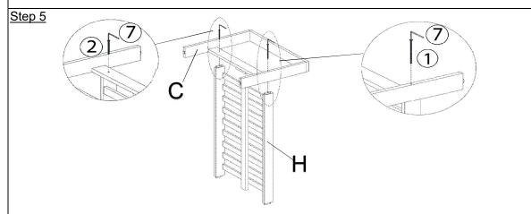
Place the Left Seat Panel (H) upright as shown in the picture above onto a clean, soft surface to avoid any scratches or damage to the product.
