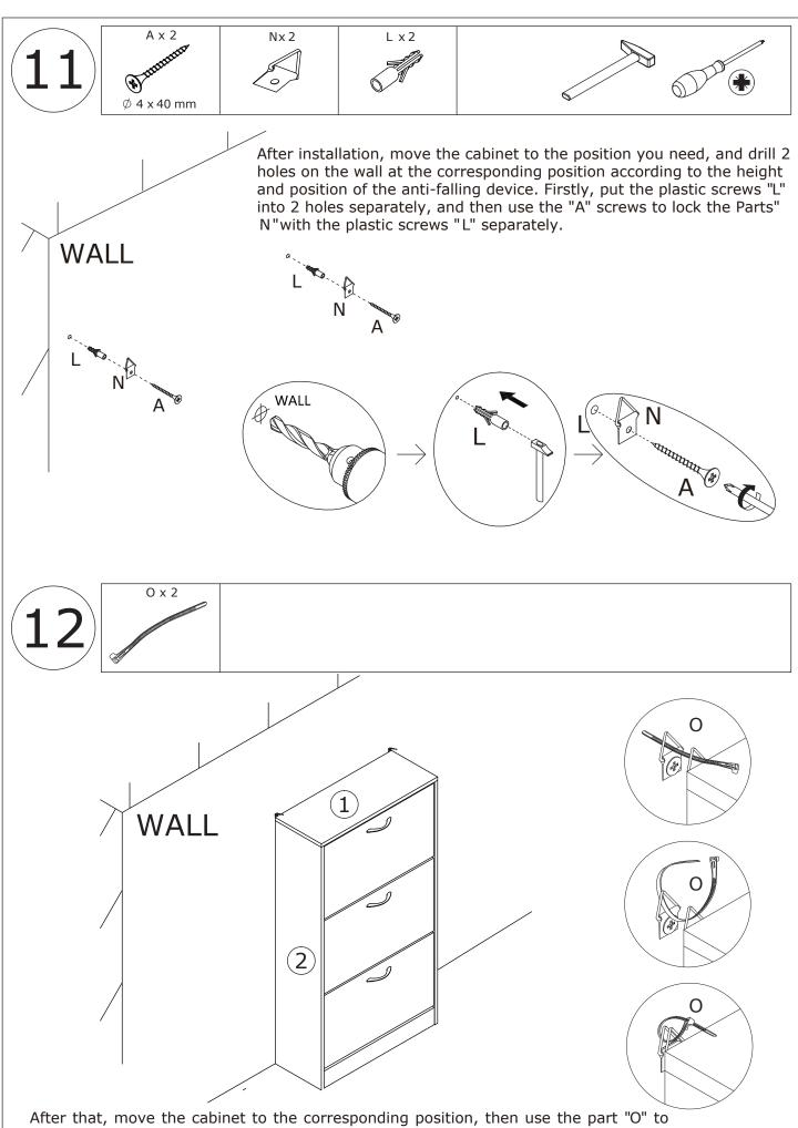
After that, move the cabinet to the corresponding position, then use the part "O" to pass through the part "N", and tighten it. The installation of the anti-falling device is completed. 11/11
