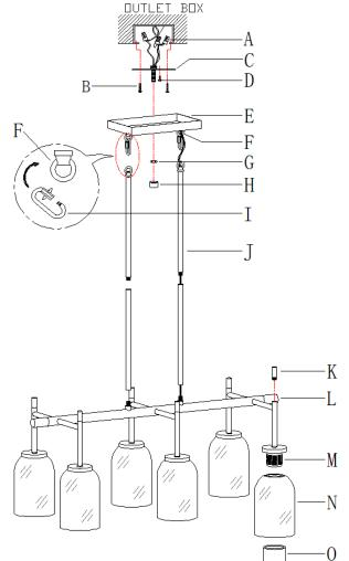
Step A1: Pass fixture wires through tubes (J), and tighten tubes (J) onto fixture body (L). Screw tube bolts (K) onto fixture body (L).
