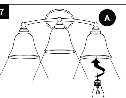
Use 60-watt max. standard-base incandescent bulbs or CFL/LED equivalent.
