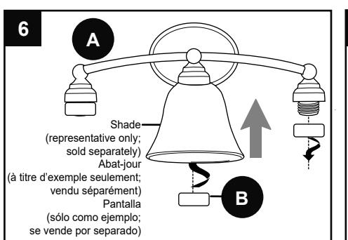
**! Do not overtighten B as shade may crack or break.**
