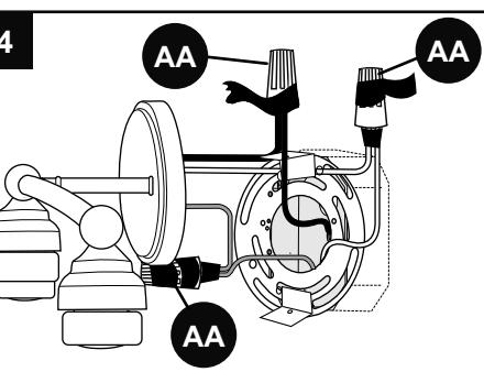
**! Make sure outlet box can support the weight of the fixture.**
