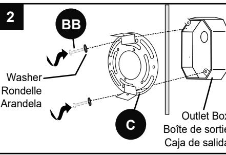
**! Make sure ears are level vertically before tightening BB.**
