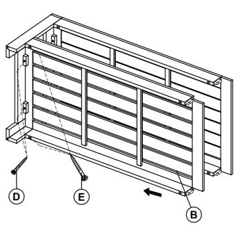
Attach the top frame (A) to the leg side frame (C). Secure using 1 1/4" screws (D) on the top frame first and tighten screws using a Phillips screwdriver. Next, secure using 2" screws (E) on the leg side frame (C) and tighten all screws using a Phillips screwdriver.
