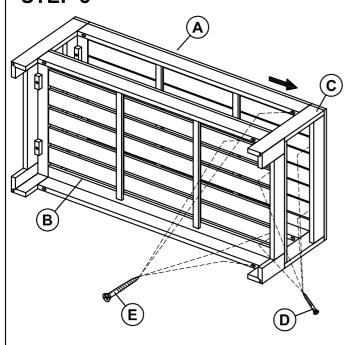
Attach the leg side frame (C) to the previous assembly. Secure using 1 1/4" screws (D) on top frame (A) and the tray frame (B) Tighten screws using a Phillips screwdriver. Next, secure using 2" screws (E) on the leg side frame (C) and tighten all screws using a Phillips screwdriver.
