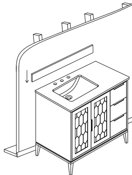
Finally,place the bottom side of back splash with sealant onto the counter top and check alignment of back splash.
