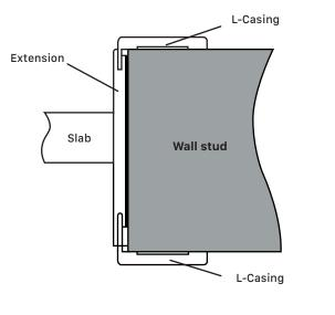
3) Discount Hardware DirectLLC Standard pocket, by-fold and bypass installation manual
