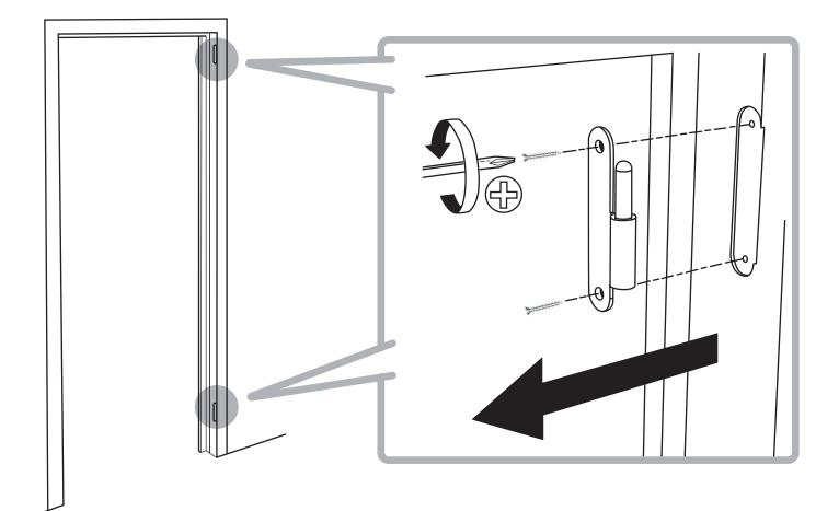
3) Please, hang the door, after hardering for construction foam. Please note: diffrent construction foams has diffrent hardering level. Read carefully the construction foam usage instructions!
