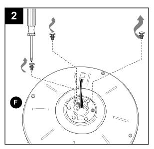
3. Pull wires up through hole in the middle of the canopy (B) and attach canopy (B) to motor (F) using the three previously removed screws/lock washers.
