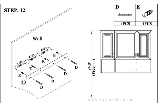
Draw the spacing between the walls and the No.10, punch holes in the wall, and fix the No.10 to the wall with screws.
