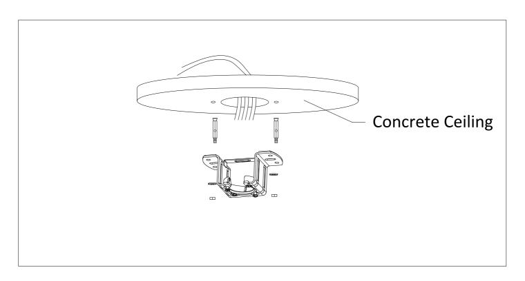
Please drill  $\phi 8$ mm hole on the concrete ceiling, and insert the bolt. Align bracket with the hole, then tighten with nut.
