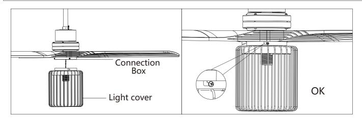
The lampshade is paired with the two lamp lines on the junction box, and pay attention to distinguish the male and the female terminals.
