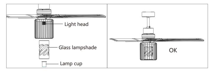
Unscrew the lamp cup from the lamp head first, then put the glass lampshade, and tighten the glass lampshade with the lamp cup.
