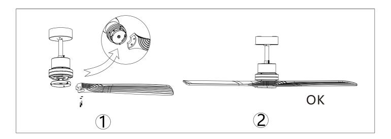
Time Saver:washers for blade screws can be set on each blade screw prior to installing blades
