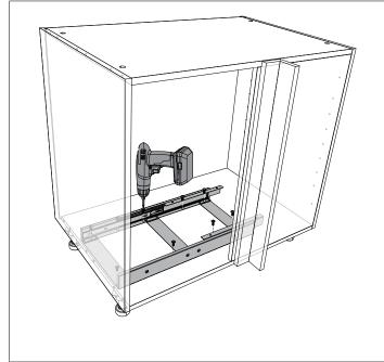
Insert the top frame assembly and align the bracket holes with the holes on the sliding base. Using a screwdriver or cordless drill fasten the top frame assembly using the eight M5x8 screws included with the assembly.
