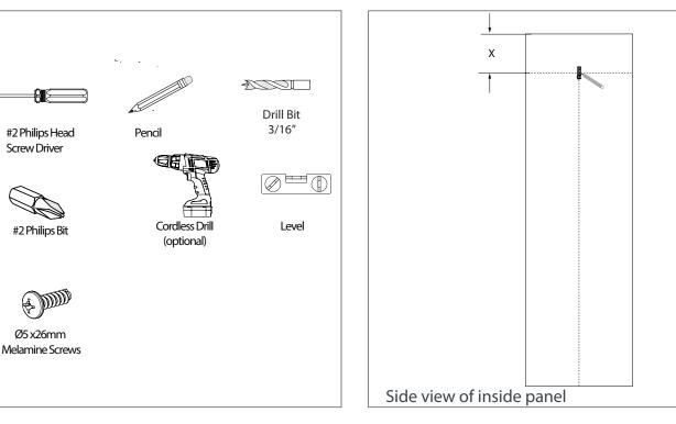
Drill holes at the marked locations on both walls using 3/16" drill bit.
