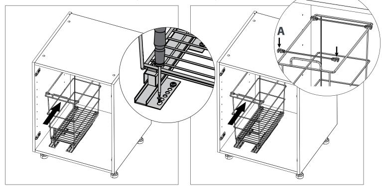
Slide the metal basket out and insert the bin. Adjust the cross posts to secure garbage bin.
