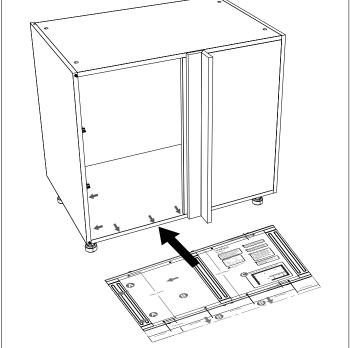
Mark the drill holes layed out on the template.
