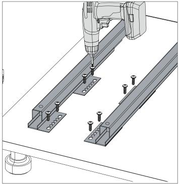
Slide the centre frame assembly onto the rails by pushing it under the clips at back of the slides as shown in (**A**). Secure front portion of the frame to the rails using two M4x6mm screws as shown in (**B**).
