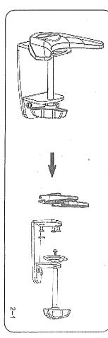
2.Re-install the base plate with three retained attach screws, tighten these screws with a 4mm allen key and paste the rubber pad on the one screw as shown on 2-2
