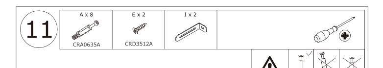
Screw eccentric rod(A) into part 1 as shown. Fix part(I) to part 1 using screw(E) as shown.
