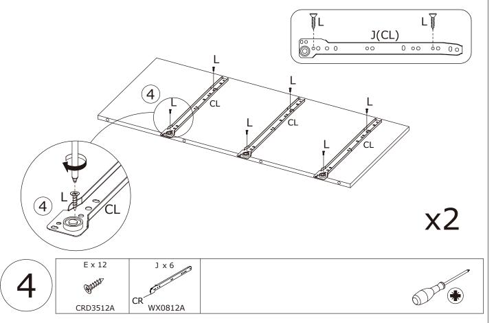
Fix slide rail(CR) to the left side of part 4 using screw(E) as shown. Please note, the pre-drilling of the rail on the right and left of this board is asymmetrical. Please install the rails according to the picture.
