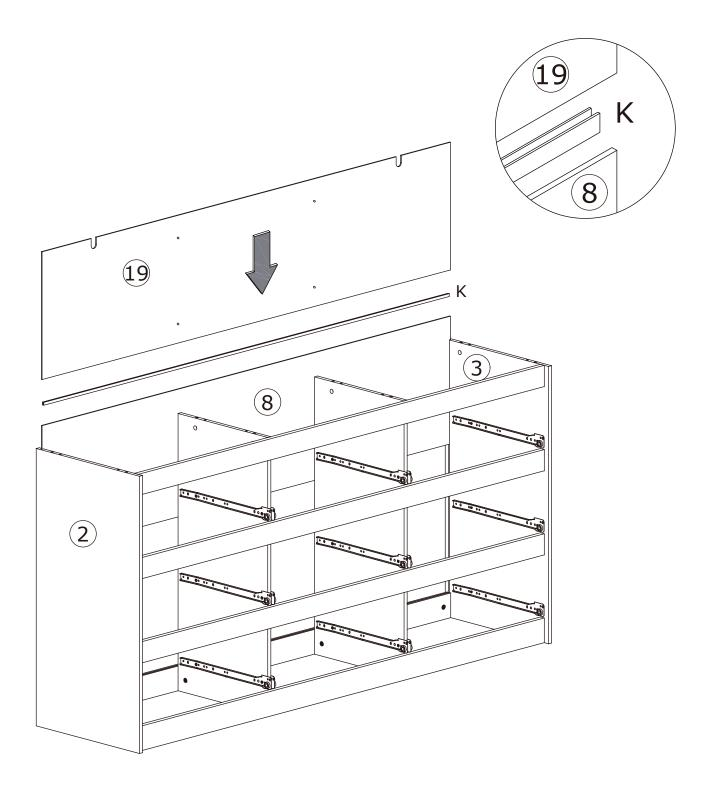
Connect part 19 and part 8 with part (K) and insert along the available slots of part 2, 3 and 7 as shown.
