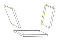
Arrange vertical zBoard with grooves facing backboard as shown.
