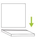
Fit backboard into horizontal zBoard groove.
