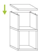
Align horizontal zBoard and press firmly to secure unit together. Visit links below for more details.
