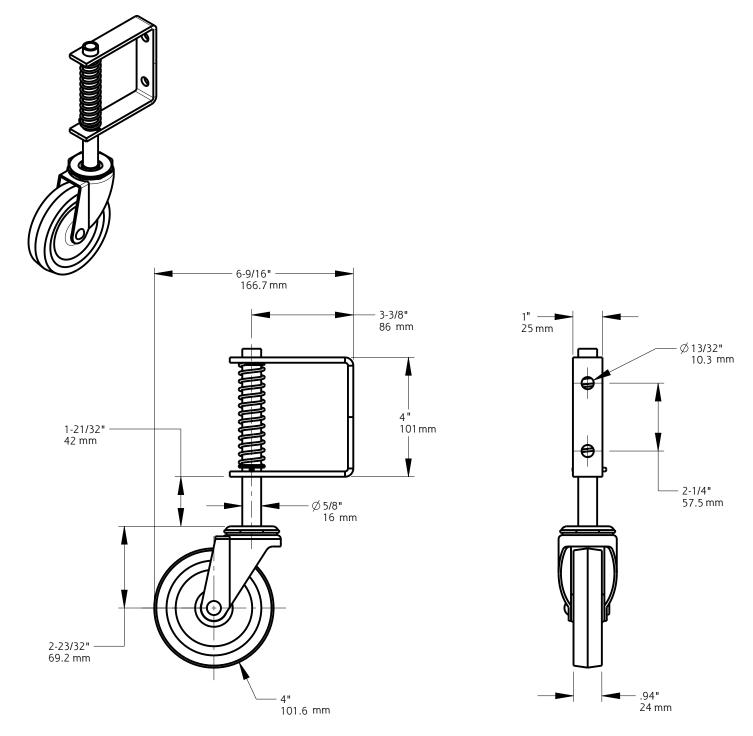
Material: Steel with hard plastic wheel Finish: Zinc Plated
