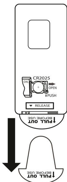
The remote control operates on one CR2025 battery (included). To activate the remote control, remove the insulation tab inserted in the battery compartment.
