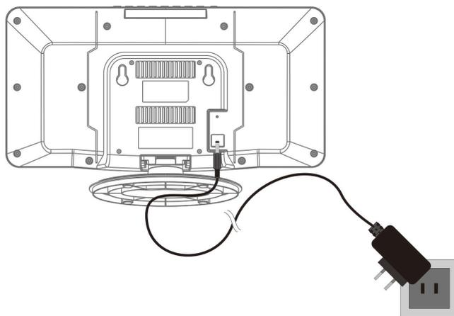
To do this, place the connection cable plug in the socket DC IN and the supplied mains adapter into a properly installed earthed power socket which is accessible at all times
