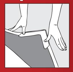
Firmly press curl stop to the problem corner of the rug. When properly installed curl stop is not visible under the rug corner when the rug is laid flat.
