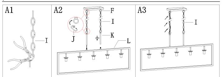
Step A1: By measuring, determine the correct number of links needed for proper hanging height. Using the chain pliers, disconnect and discard the unwanted part.
