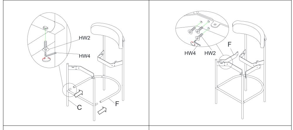
**Step3:** Insert the tenon on Front leg "C" into stretcher "F", and then assembly (not tighten) by HW2,
