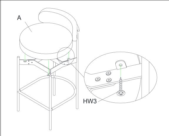
**Step5:** Place the chair onto even floor and then tighten all Bolt,
