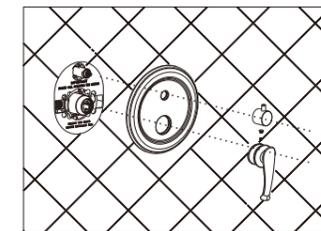
According to the figure below, please correctly adjust the direction of water separator handle
