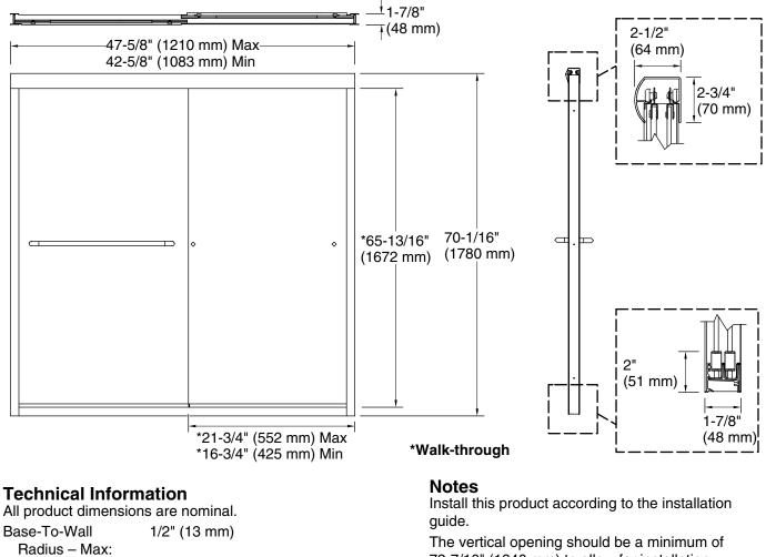
Shower Ledge Min 2-1/8" (54 mm) Flat: Shower Wall Min 2-11/16" (68 mm) Flat: The vertical opening should be a minimum of 72-7/16" (1840 mm) to allow for installation clearance.
