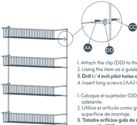
1. Attach the clip (DD) to the item; clamp the wire with the opening of the clip and push it forward.
