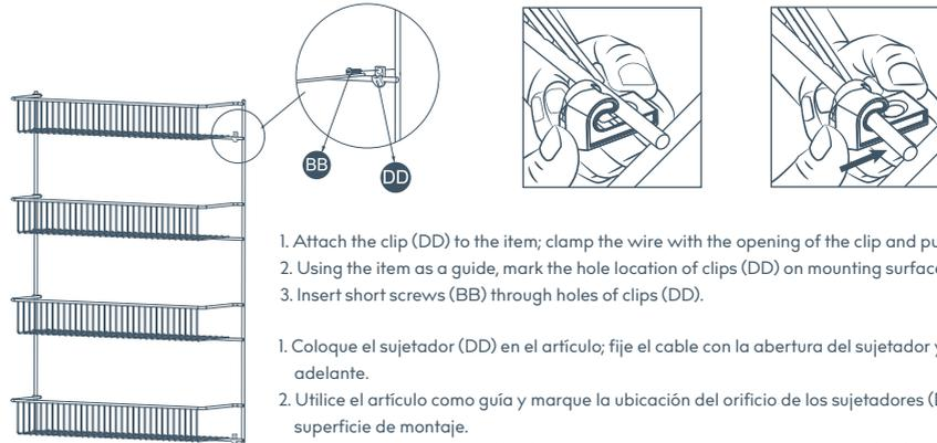
1. Attach the clip (DD) to the item; clamp the wire with the opening of the clip and push it forward.
